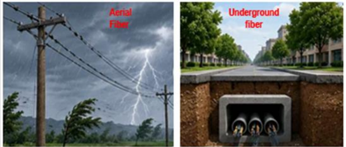
Figure 3: Aerial versus Underground Fiber Deployment 4
